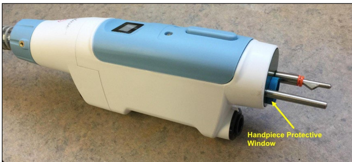
Figure 5-12. Handpiece protective window is located inside the snap-in holder between distance gauges.
